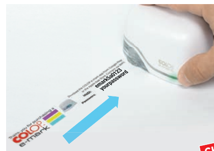
11. Print a test image and compare it to the imprint below to verify quality
